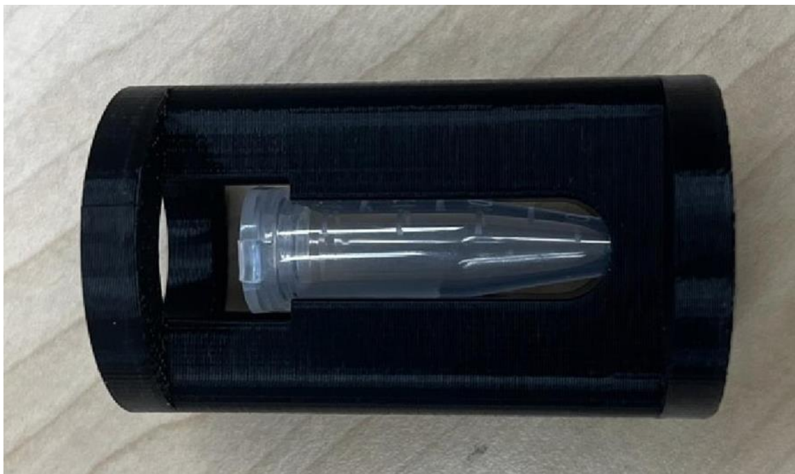
Figure 3-4. 3D printable adapter for microcentrifuge tube.
